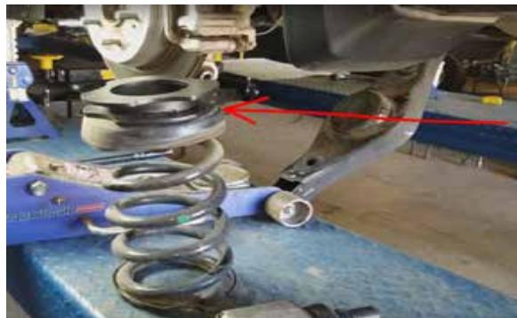
Place spacer on top of rubber isolator. Ensure the notch aligns correctly.
