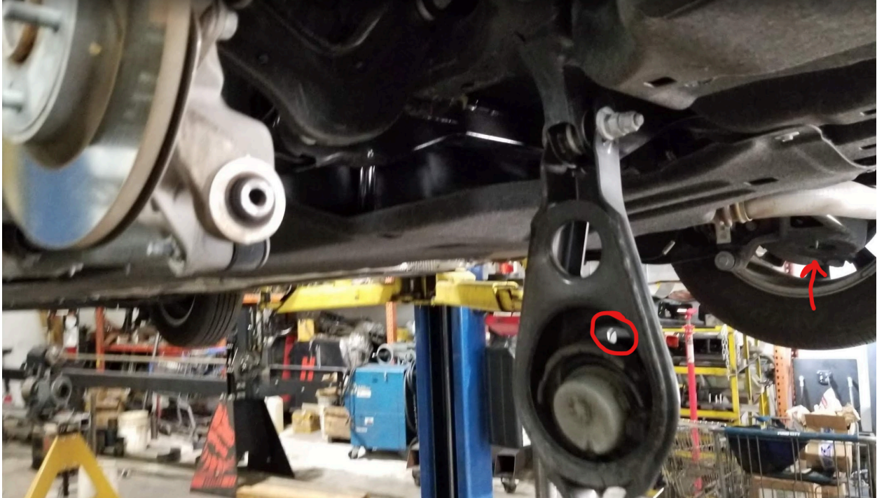
Rear Suspension arm hanging down. Stud goes through red hole
