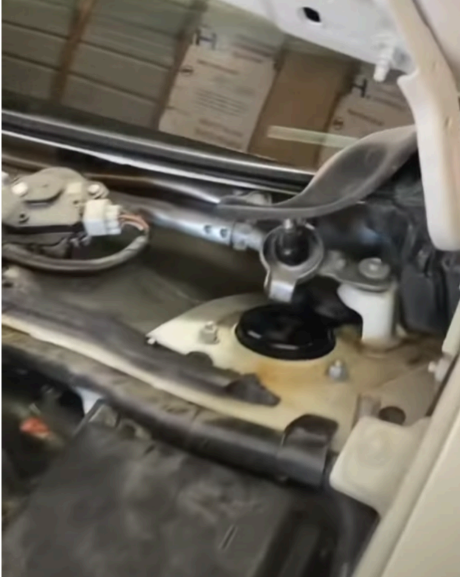
Front strut mount with windshield wiper cowl removed
