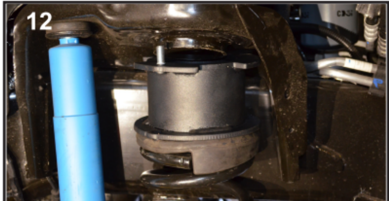
12 Fit the stud on the top of the spring spacer into the hole in the spring perch. Use a 10mm nut on the stud to secure.
