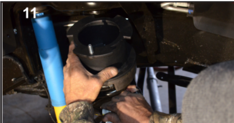
11 Reinstall spring into truck, ensuring proper alignment of spring, isolator, and spacer.
