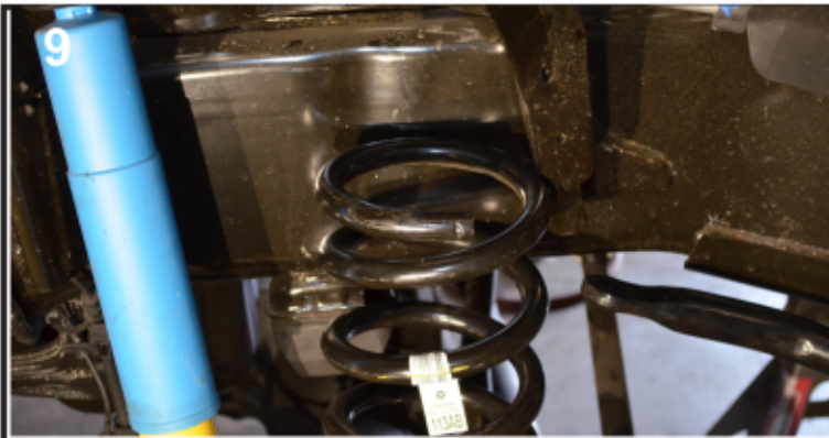
9 Remove coil springs. Take note of the direction that the rubber isolator and spring are facing for proper reinstallation.
