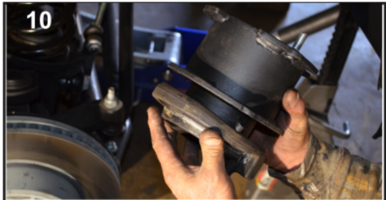
10 Install rubber spring isolator onto the base of the new 3.5" Traxda coil spring spacers. Place on the top of the coil spring.
