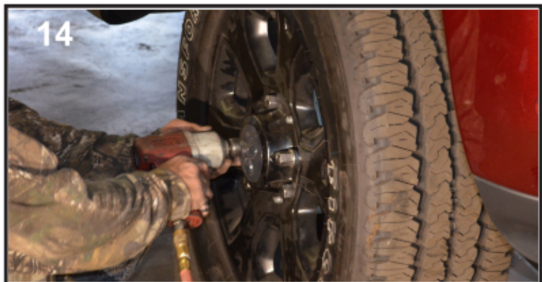
14 Reinstall wheels if removed. Make sure to double check all work. Center steering wheel, it will have moved during installation.
