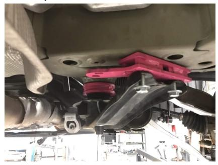
16. Install new bolt on steering shaft - the shallow bolt will prevent rubbing on
