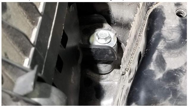
19. With strut removed, install Traxda preload spacer 32.5 using a strut compressor. DANGER! Strut compressors have a lot of pressure and can be dangerous! Use a quality strut compressor!
