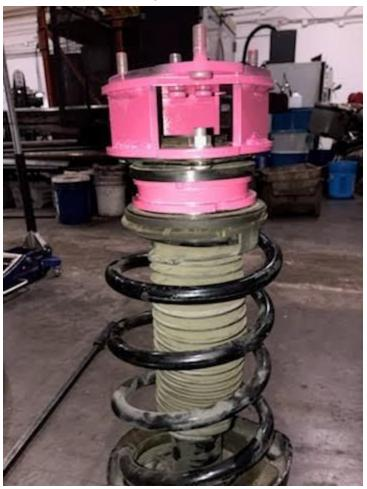
21. Leave camber adjustment loose for now. The arrow on Traxda Strut cap 34.1 faces forward. Right and Left sides of truck use the same part.
