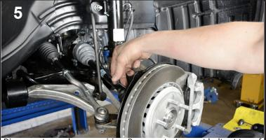
Disconnect speed sensor wiring. Remove strut mount bolts at top of strut, behind plastic cover. Remove lower strut mount bolt.
