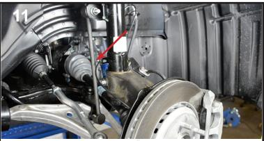
Install strut into spindle, using 36" prybar on lower control arm. Install Traxda replacement sway bar link, discard original links.
