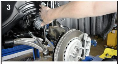
Remove sway bar links and ball joint.
