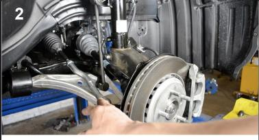
Remove brake caliper and disconnect tie rod.
