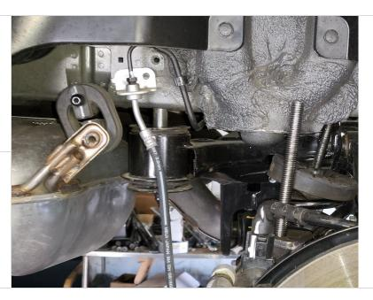
loosen the sway bar bushings. They are very tight on this vehicle
