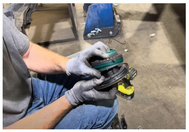
9. Reattach the black metal top to the strut, compress springs more and reattach the top nut.
