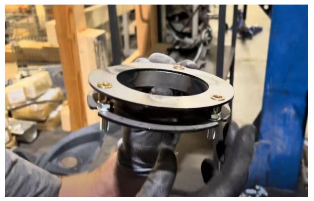
12. Reinstall strut to vehicle, loosely tightening the three OEM bolts into the top for now.
