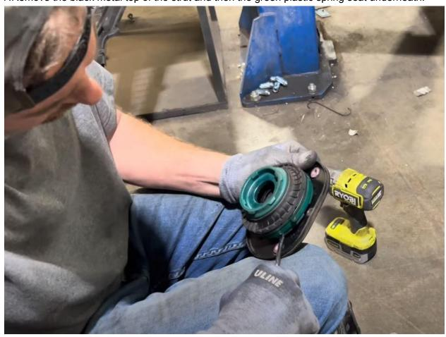
8. Attach the TRAXDA preload spacer under the green plastic spring seat, lining up the pin.
