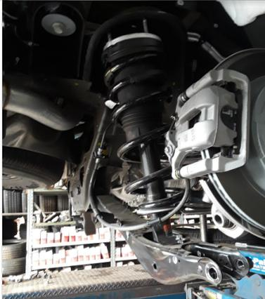
Install plates on top of strut and reinstall using supplied nuts
