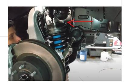
Install plates on top of strut
