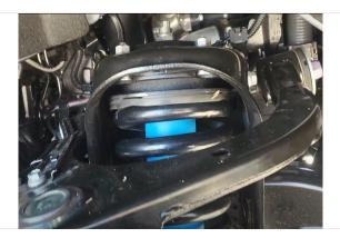
remove bump stop and install washer on bump stop, reinstall
