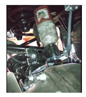
remove brackets for brake lines at differential
