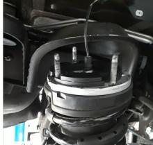
Install plates on top of strut and reinstall using supplied nuts
