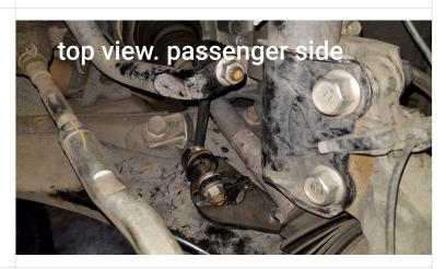
11. Install the supplied sway bar links (same as rear) to new mount. The links have a RIGHT and LEFT to them, make sure they are on the correct side.
