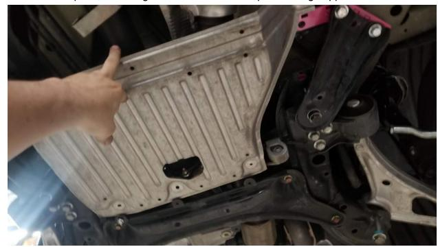
34. Reinstall skid plate, attaching to subframe bracket spacer using supplied bolts.
