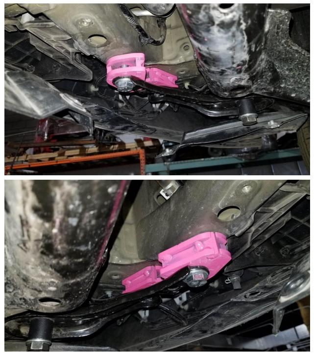
28. Install subframe bracket spacer 33.20 at rear corners of subframe. Tab with hole in it should be away from the body.
