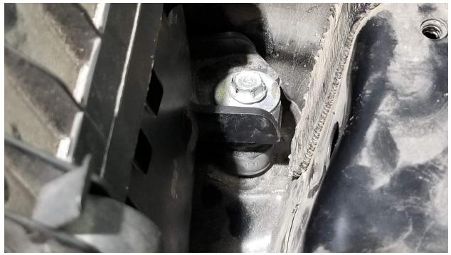
19. With strut removed, install Traxda preload spacer 32.5 using a strut compressor. DANGER! Strut compressors have a lot of pressure and can be dangerous! Use a quality strut compressor! 20. Install Traxda strut cap 34.1 onto reassembled strut.
