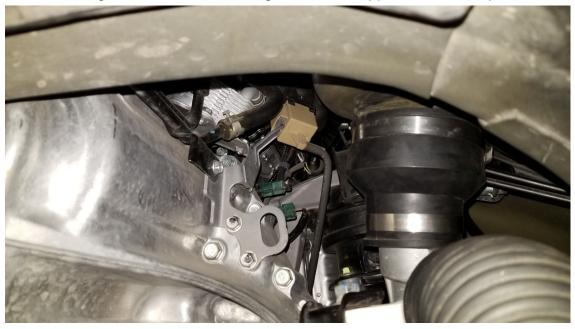
18. Remove and re-install airbox mount at back of box. Relocate rubber bushing to beneath airbox mount tab. This will change the angle of the airbox to correct for subframe drop. The back of the airbox should be angled up.
