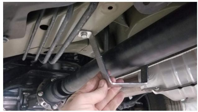
36. Install drive shaft spacers 33.25 and 33.26 under the steady bearings using supplied bolts. Trim plastic skid plate to fit around bolt.
