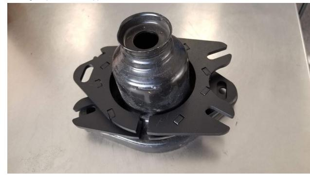
c. Ridgeline rear will mount properly with small gap. Pilot rear will mount properly with no gap.
