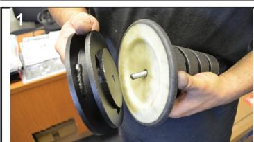
Take Traxda Spacer and install onto bumpstop, pushing bolt through hole.
