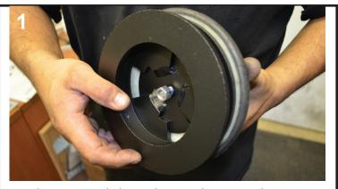
Tighten nut onto bolt, attaching Traxda Spacer to bumpstop.
