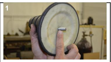
Bolt should extend out of top of bumpstop.
