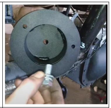
Attach Traxda part to differential with supplied 8mm bolts and nut
