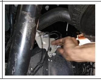
Drop the axle remove the 2 bolts from the bags, lift the airbags
