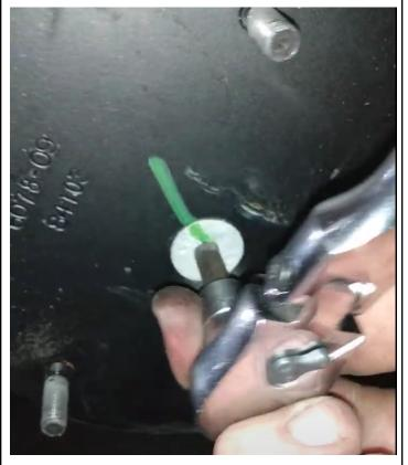
Install Traxda part with supplied 12mmx30x1.75 bolt and use lock washer and plain washer.
