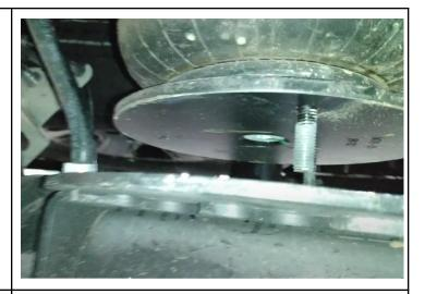
Remove Hex bolt from bottom of air bag to remove lower plate.
