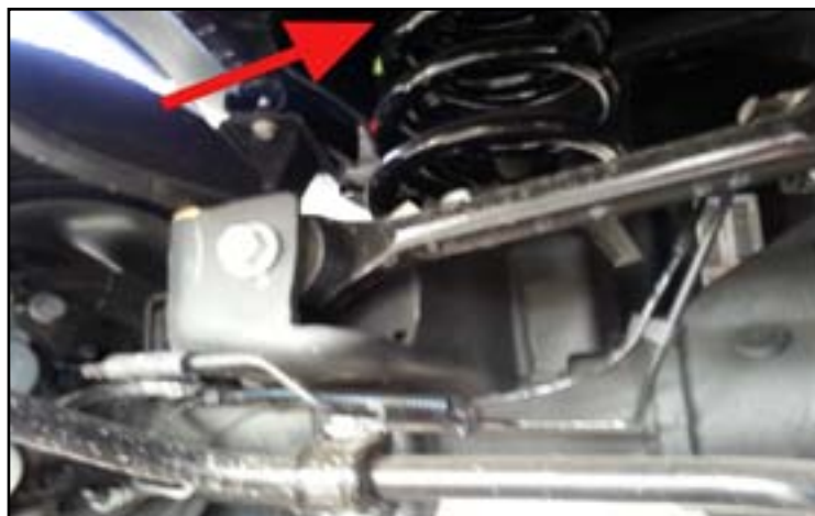
Rear - 1 Raise rear of vehicle and support with jackstands at frame on both sides. Remove wheels, support axle on one side and remove the lower shock mounting bolt.
