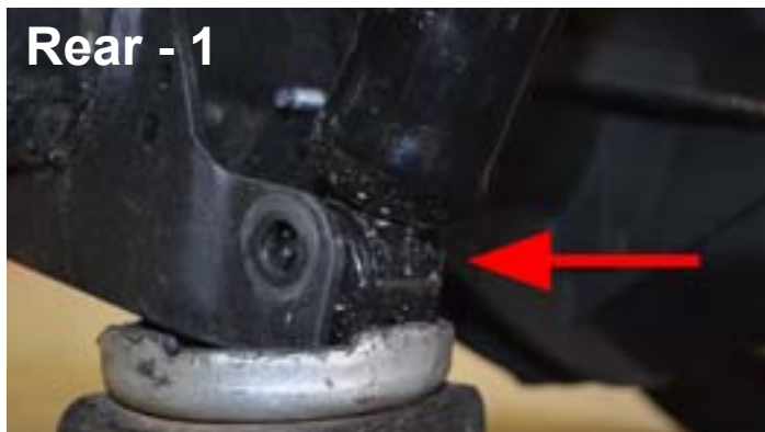
Rear - 1 Raise rear of vehicle and support with jackstands at frame on both sides. Remove wheels, support axle on one side and remove the lower shock mounting bolt.
