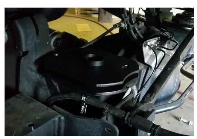
8. Use supplied bolts to fasten spacer to differential
