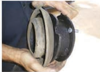
Figure A: Installing isolator pad on TRAXDA spacer
