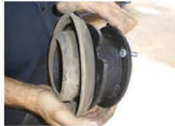
Figure A: Installing isolator pad on TRAXDA spacer
