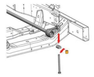
2) Install the shock extensions using supplied hardware. NOTE: Shock extensions are not used in the Chevrolet Colorado or GMC Canyon.
