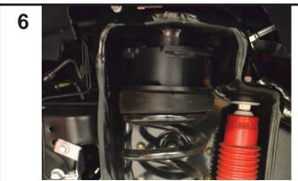
Re-install spring and spacer. Repeat step 5 on other side. Raise axle with jack until springs are seated.
