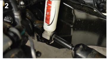
Support the front axle with a jack. Disconnect the lower shock mounts at both sides.
