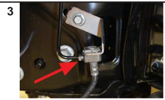
On both sides, remove stock brake line bracket and replace with Traxda bracket. Attach brake line as shown above. You will need to loosen the brake line at the hardline junction and rotate 180°.
