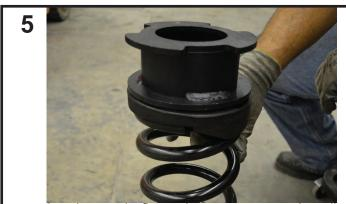
Lower the axle using the floor jack. Remove spring and install Traxda Spacer as shown above.
