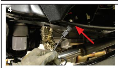
On both sides, disconnect the ABS line at frame.
