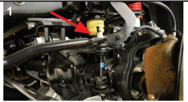
Raise the truck with a jack and place on jack stands at the chassis. Remove wheels and tires. Disconnect sway bar link at the sway bar on both sides.
