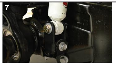
On both sides, install Traxda Shock Extensions to shock using supplied hardware. Install Extensions to axles using OEM hardware.
