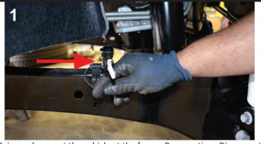
Raise and support the vehicle at the frame. Remove tires. Disconnect ABS lines at the body mount behind the front fender cover.
