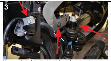
Disconnect brake hose brackets at front of spring perch and up on frame. Disconnect sway bar link.
