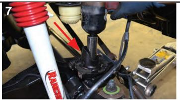
Using supplied hardware, bolt down the spring perch and Traxda Spacer. Reinstall spring, raise axle and reinstall lower shock mount bolt.
