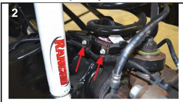
Disconnect two ABS wire mounts from backside of spring perch.
