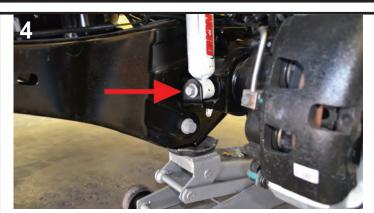
Supporting the axle with a jack, remove the lower shock mount bolt. Slowly lower the jack until the spring becomes free. Note the spring orientation for re-installation.
