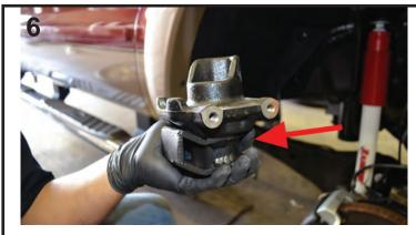
Fit Traxda Spacer underneath spring perch.
