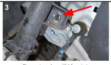
Disconnect sway bar end link from strut.
