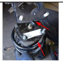
Install spacer on strut using factory nuts. Align notched edge with curved edge of strut mount. Reinstall in vehicle with curved edge facing away from engine.
