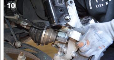
Reinstall lower strut mounting bolts while guiding axle through the spindle. Tighten all strut nuts fully, upper and lower.
