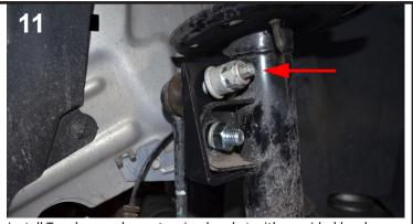
Install Traxda sway bar extension bracket with provided hardware.
