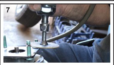
Cut 0.25" from the top of the mounting studs on the upper strut.
