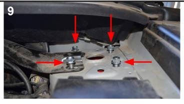
Reinstall upper strut mounting nuts. Do not tighten fully.
